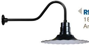
▶ R918-41-E6-41-200GLFR-GUP-41-RTC-42WPL-41 18" Radial Shade with 200W Frosted Glass, Wire Guard, E6 Arm in Black and RTC Ballast Housing with Fluorescent Ballast. Fluorescent ballast accommodates 26WCFL, 32WCFL, or 42WCFL.
