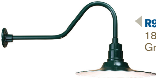
▶ R918-42-E6-42-200GLFR-GUP-42-RTC-42WPL-42 18" Radial Shade with 200W Frosted Glass, Wire Guard, E6 Arm in Forest Green and RTC Ballast Housing with Fluorescent Ballast. Fluorescent ballast accommodates 26WCFL, 32WCFL, or 42WCFL.
